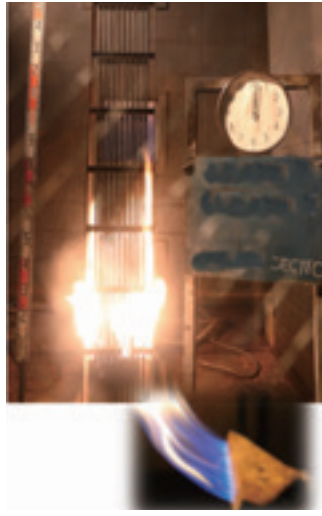
Multiple cables vertical tray flame propagation test
