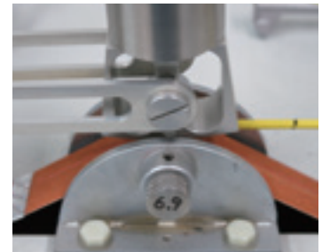
Sandpaper abrasion test
