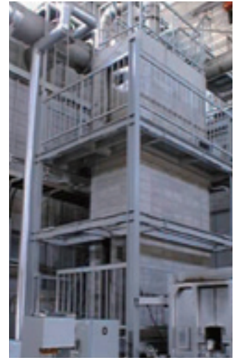
Riser cable flame propagation test
