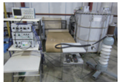
Partial discharge test
