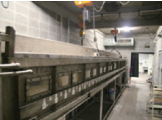
Steiner tunnel surface/cable burning test
