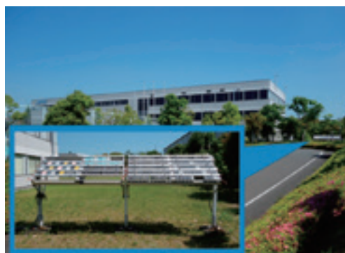
Outdoor exposure testing on JECTEC ground (Implementation of evaluations regarding changes in physical properties, external appearance of samples, and so on)
