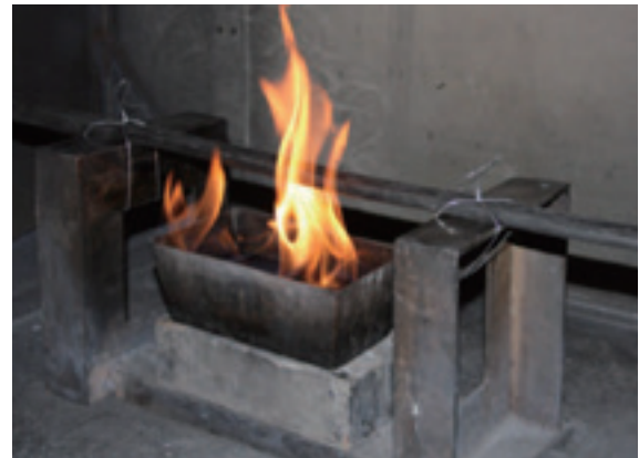
3 m cube smoke density test
