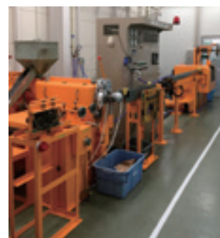
40 mm extruder at JECTEC Environment Building (implementation of electric wire trial production and evaluation)
