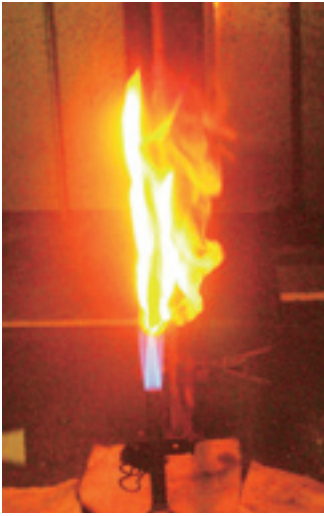
Single cable flame propagation test
